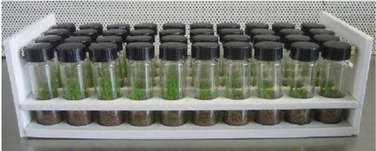
Figure 1: Turfgrass cultivars were screened inside 15 ml glass vials with grass grown on a sand base. After one to two weeks of growth from seed, defense activators were applied. After another week, grass was inoculated with ground-up grain inoculum of the brown ring patch fungus, Waitea circinata .
